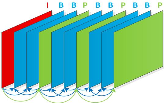
Figure 3: Frames in a H.264 stream
